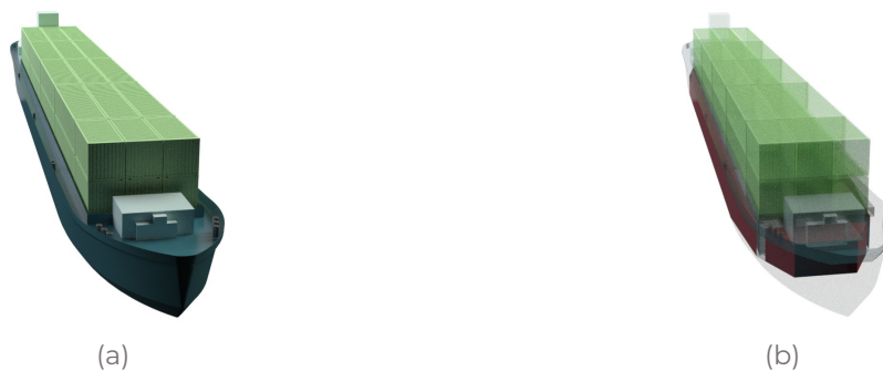
Figure 3-5: “Johann Welker” (1952) (CEMT IV reference design): a) cargo space utilization when loading containers, b) “lost” cargo space beneath the deck.
