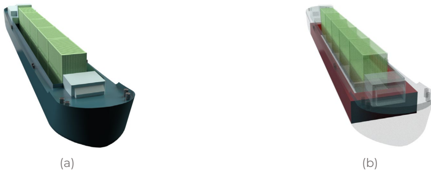
Figure 3-3: “Oskar Teubert” (1953) (CEMT II reference design): a) cargo space utilization when loading containers, b) “lost” cargo space beneath the deck.
