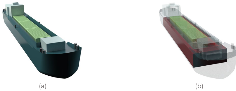
Figure 3-2: “Theodor Bayer” (1955) (CEMT I reference design): a) cargo space utilization when loading containers, b) “lost” cargo space beneath the deck.
