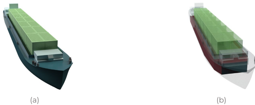
Figure 3-4: “Gustav Koenigs” (1950) (CEMT III reference design): a) cargo space utilization when loading containers, b) “lost” cargo space beneath the deck.
