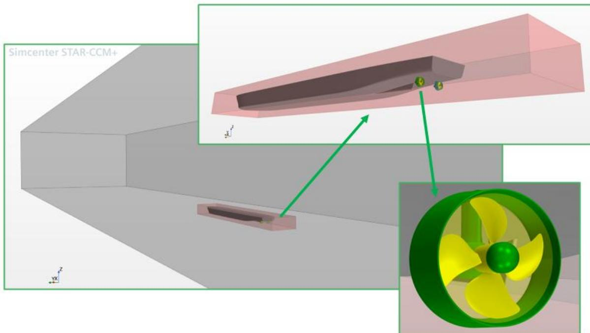
Figure 11-7: CFD Model Setup for the developed AUTOFLEX conceptual vessel design and the corresponding propulsion system
