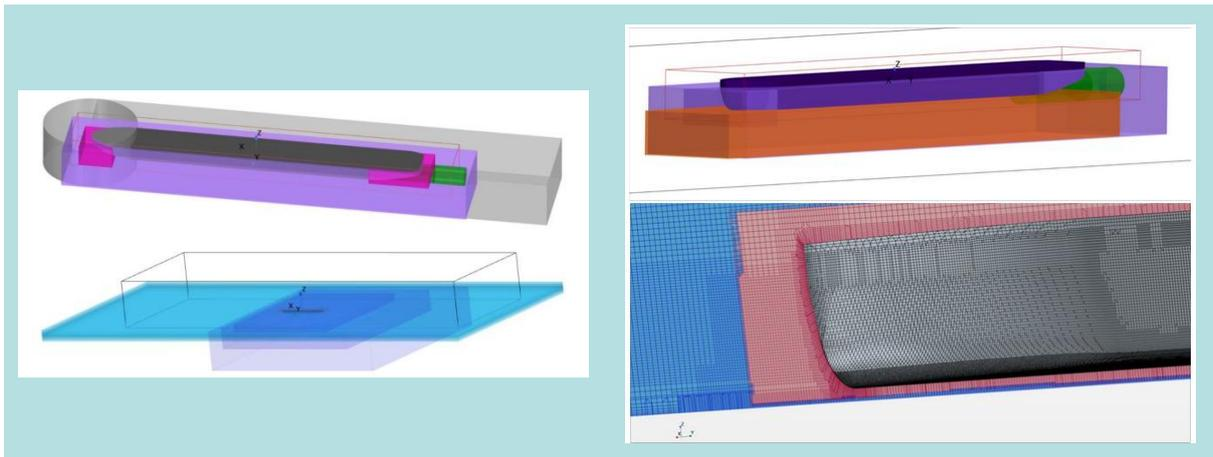
Figure 11-8: CFD Setup illustrating the standard volume refinement controls (left) and the bottom refinement control specific to extreme shallow water conditions
