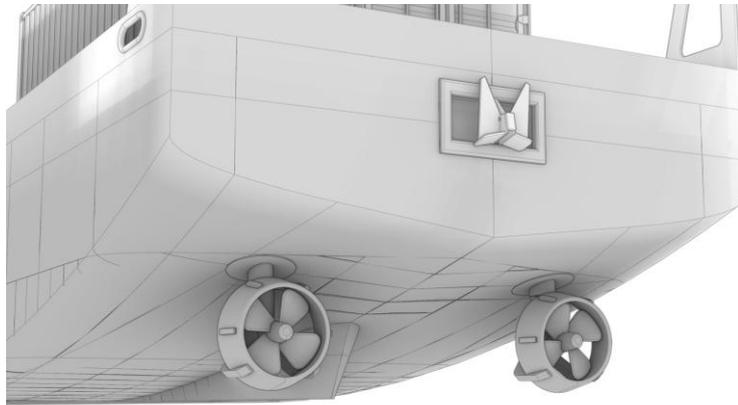
Figure 6-6: Main propulsion system. Two azimuth thrusters with total power of 380 kW and propeller diameter of 0.85 m
