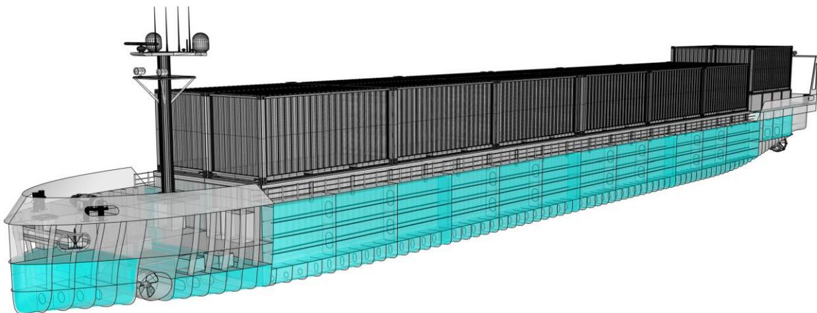
Figure 5-5: Representation of double bottom and double side structures with ballast tanks arrangement of initial design
