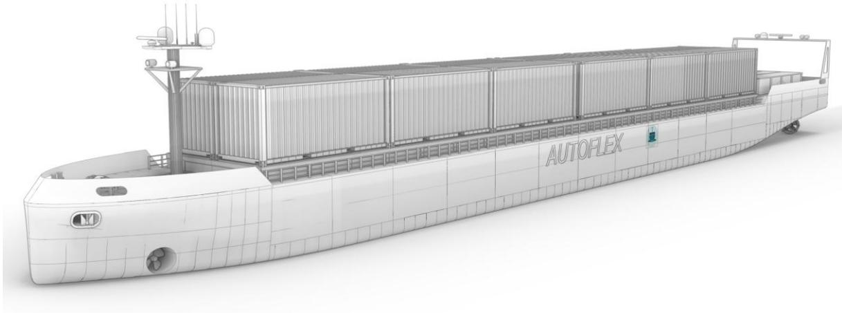
Figure 5-4: Initial design of AUTOFLEX CEMT II vessel
