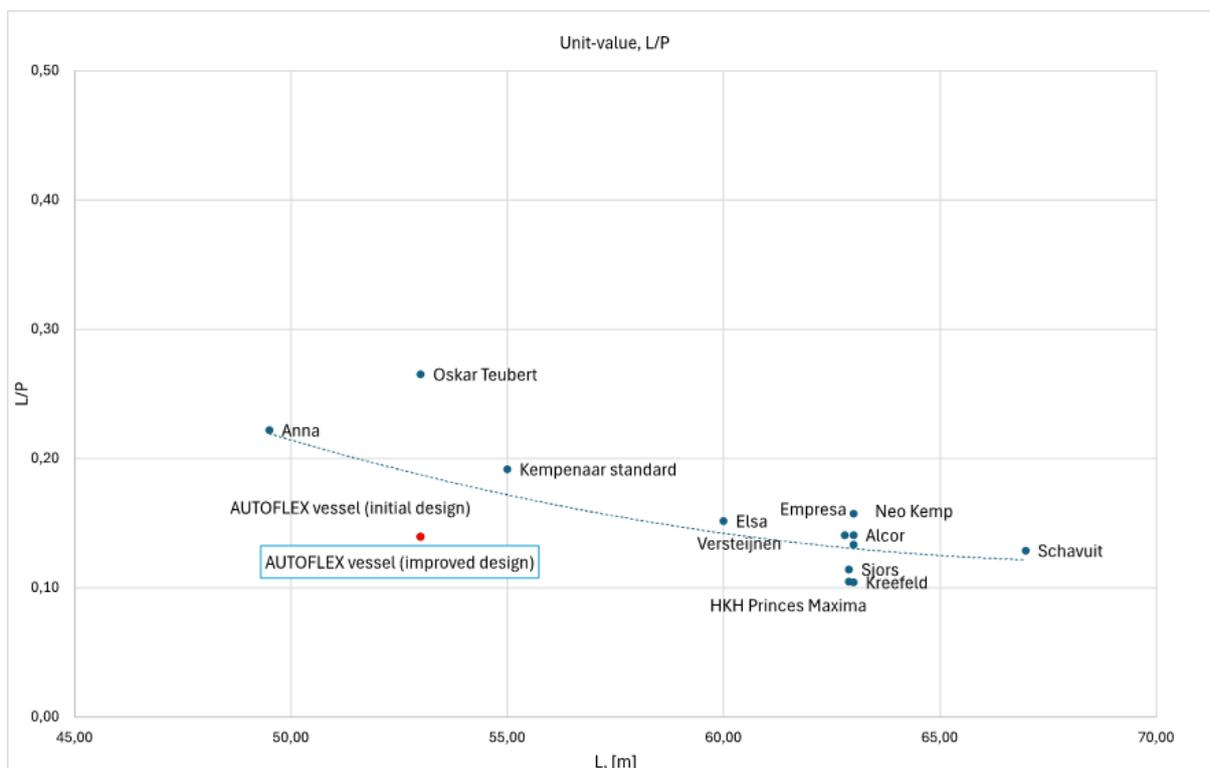
Figure 4-6: *L/P* – Length-to-Installed Power ratio
