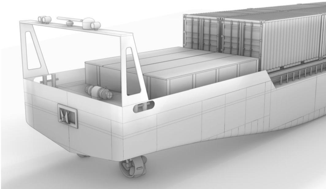
Figure 5-7: ZESpacks mounted on tween deck in enclosed compartment
