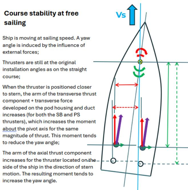
Figure 11-3: Schematic illustration of course stability at free sailing
