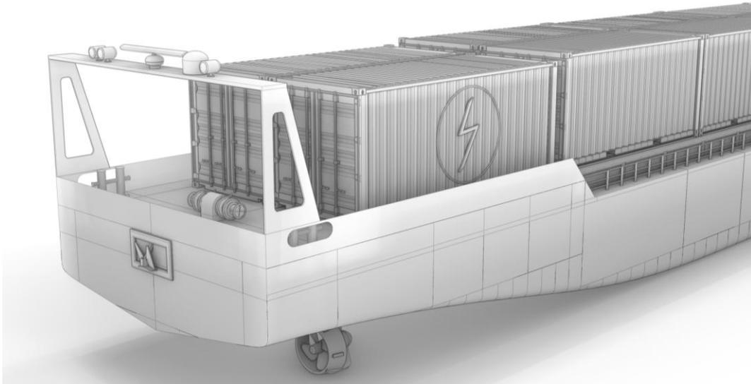
Figure 5-6: ZESpacks mounted on poop deck
