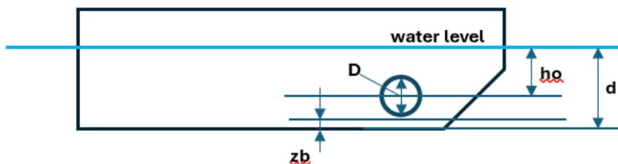
Figure 11-6: To the definition of tunnel thruster submergence
