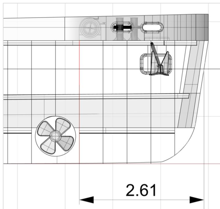
Figure 6-11: Positioning of collision bulkhead
