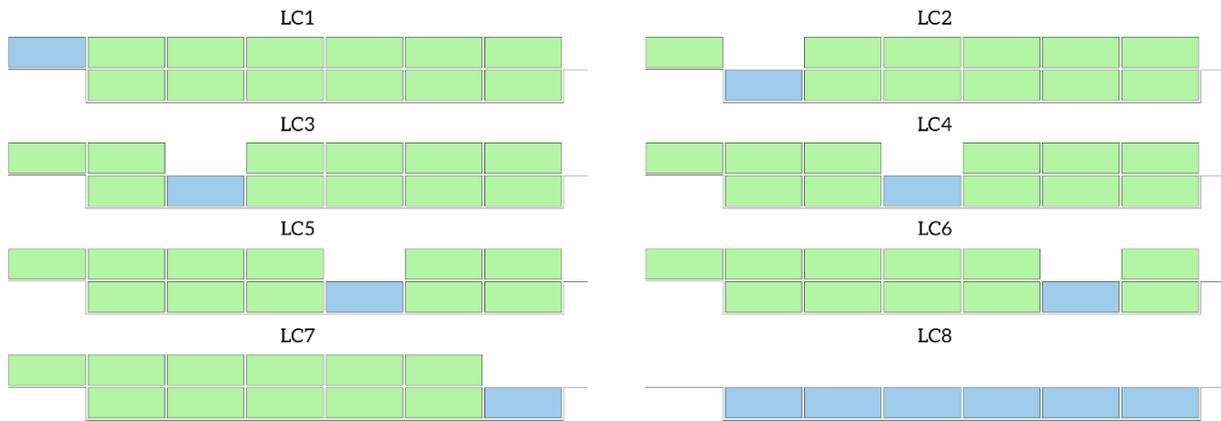
Figure 10-2: Main loading conditions considered for the stability assessment, showing different configurations of cargo containers (green) and swappable battery packs (blue)
