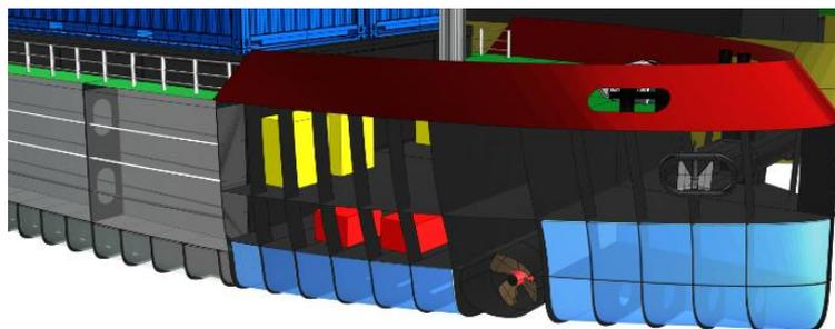
Figure 5-8: Forward ballast tanks arrangement at the bow of the vessel
