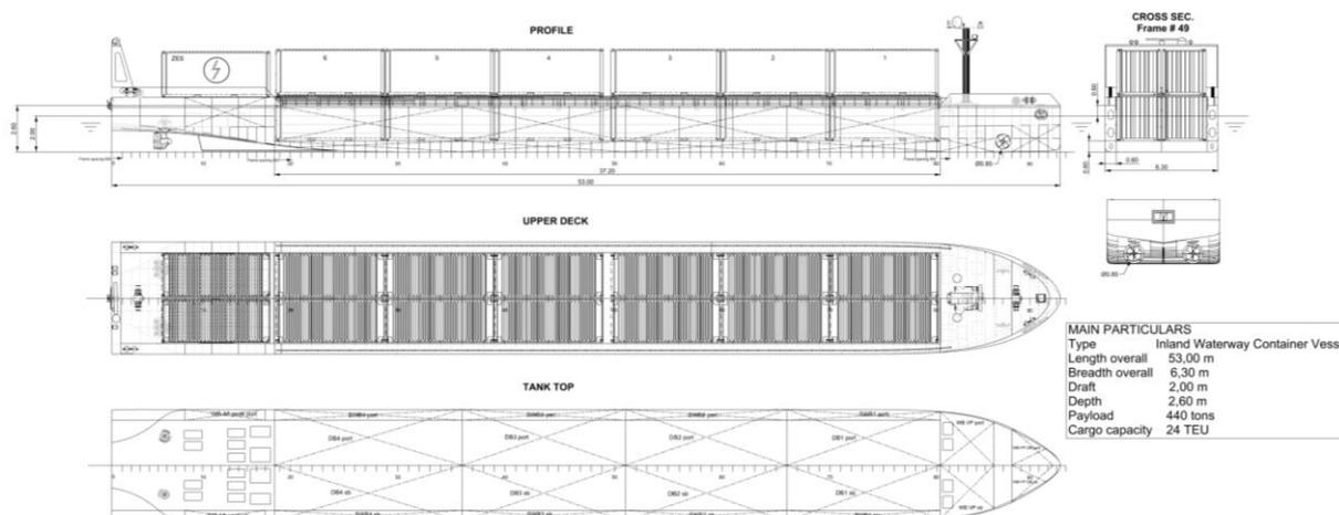
Figure 5-9: General arrangements plan of initial design of AUTOFLEX CEMT II vessel
