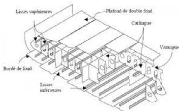
Figure 6-8: For comparison purposes: longitudinally framed double bottom [33]
