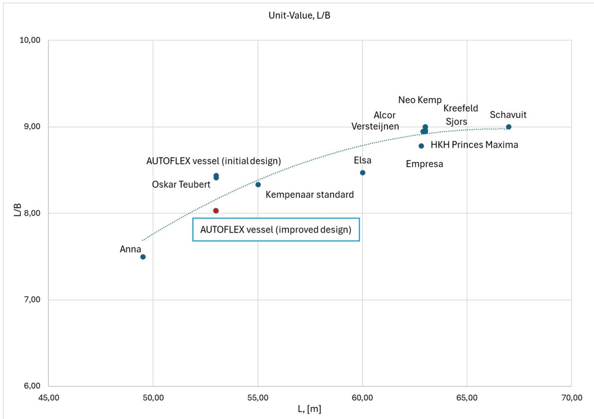
Figure 4-2: L/B – Length-to-Beam ratio
