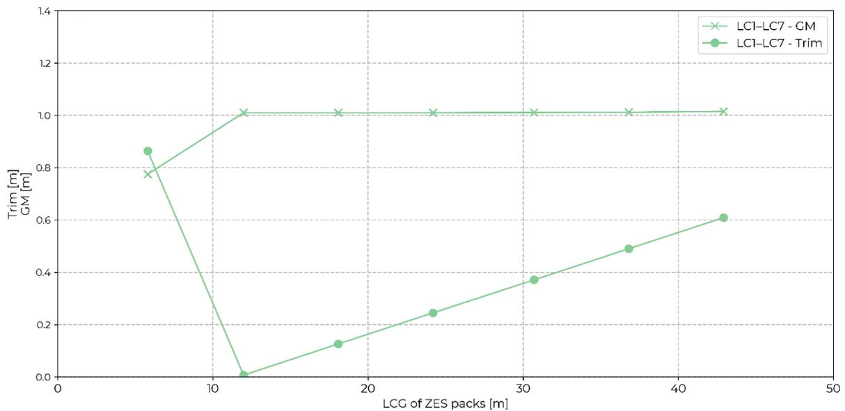
Figure 10-3: Influence of longitudinal position (LCG) of ZES battery packs on vessel trim and metacentric height (GM) for loading conditions LC1 to LC7
