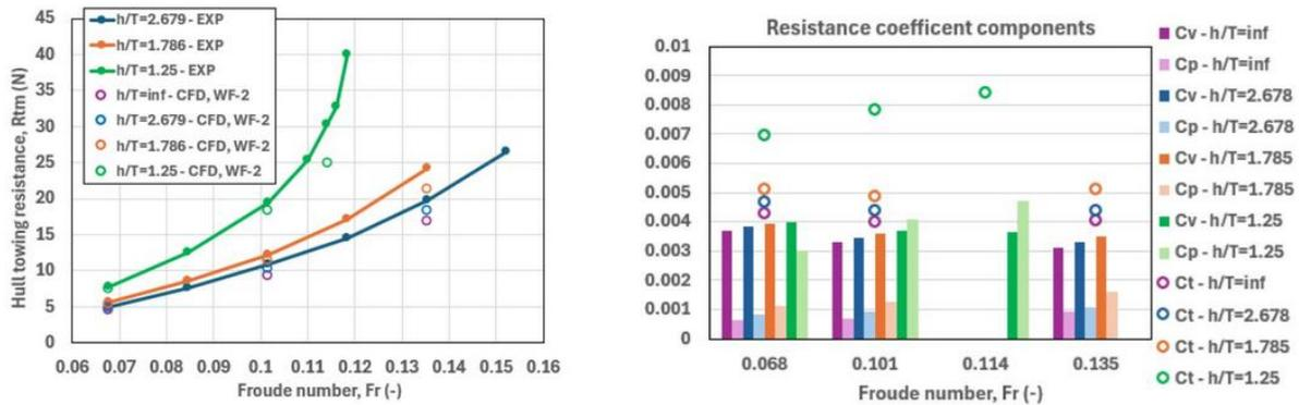
Figure 11-9: Direct comparison of the towing resistance between the CFD results and experimental measurements
