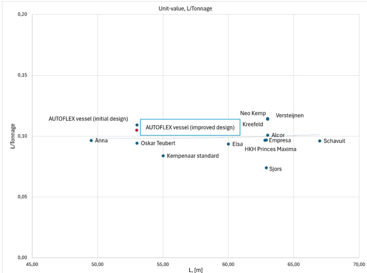
Figure 4-5: L/Tonnage – Length-to-Tonnage ratio
