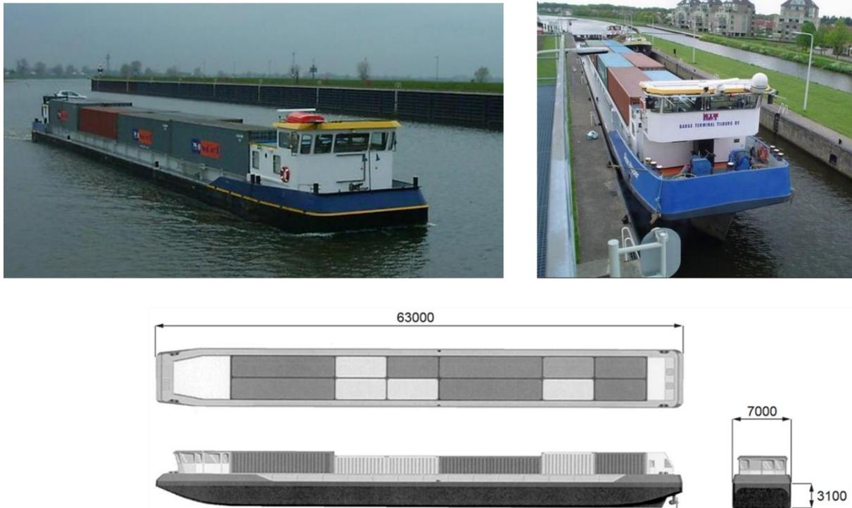
Figure 3-2: Neo-Kemp II BV: a 32 TEU inland container vessel [10], [11]
