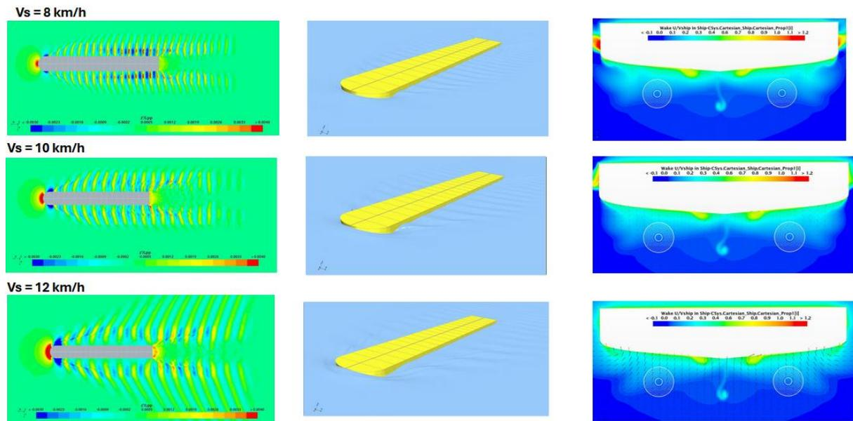
Figure 11-12: CFD simulation results of free surface waves and nominal wake fields for different service speed levels
