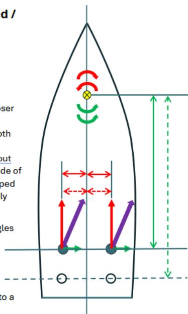
Figure 11-2: Schematic illustration of the influence of the thruster positioning at low speed
