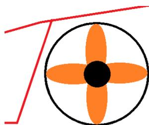
Figure 11-4: Schematic illustration of the positioning of the azimuth thruster behind the central skeg
