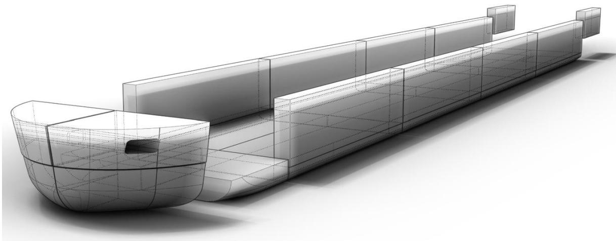
Figure 6-5: Arrangement of water ballast (WB) tanks in the vessel
