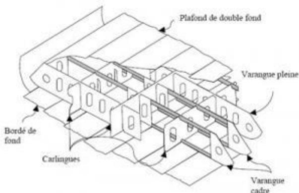
Figure 6-7: Transversely framed double bottom [33]
