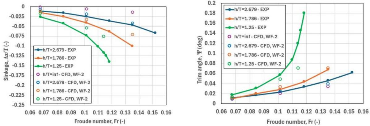
Figure 11-10: Direct comparison of the dynamic position between the CFD results and experimental measurements
