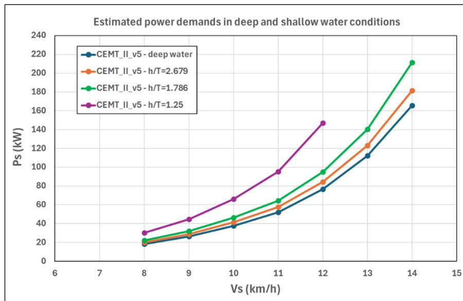
Figure 11-13: CFD simulation of estimated power demands in deep and shallow water conditions
