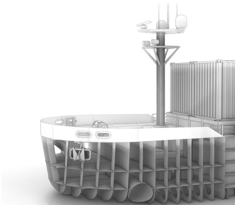
Figure 6-1: Fore-section of the vessel
