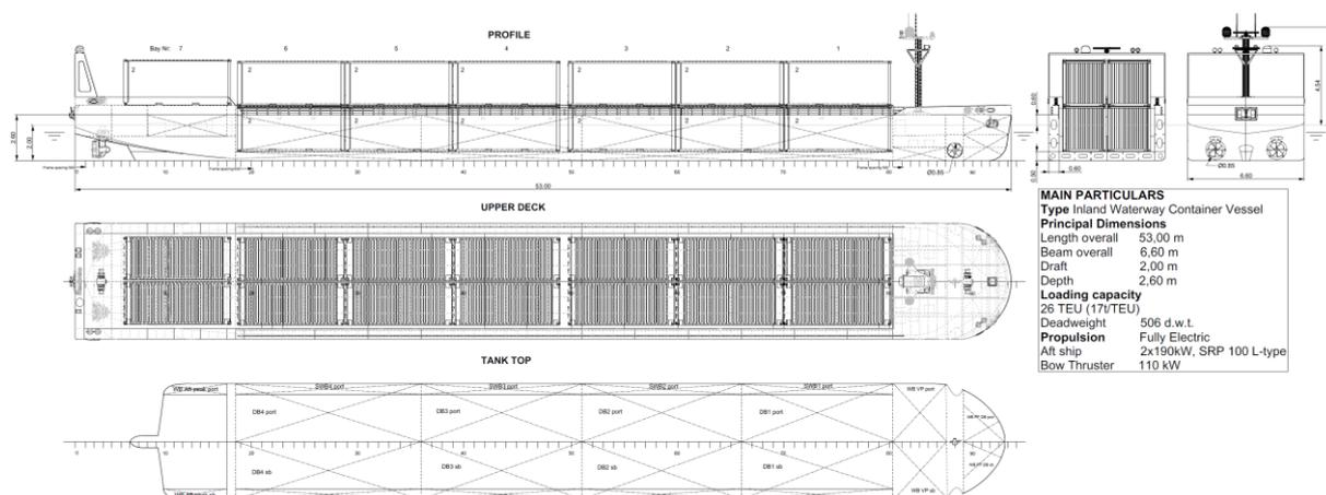
Figure 9-1: GAP of AUToFLEX CEMT II vessel
