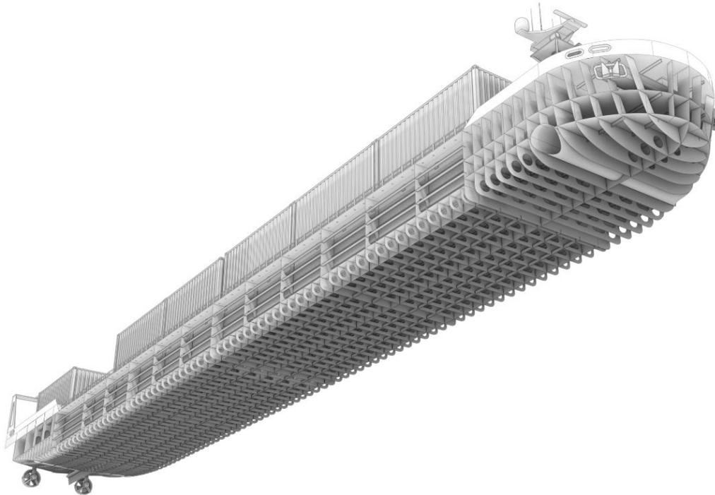
Figure 6-4: Double-bottom and double-side structures of the vessel
