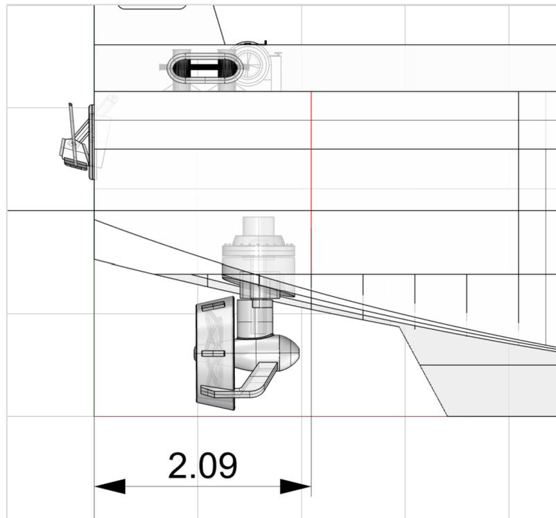
Figure 6-12: Position of aft-peak bulkhead
