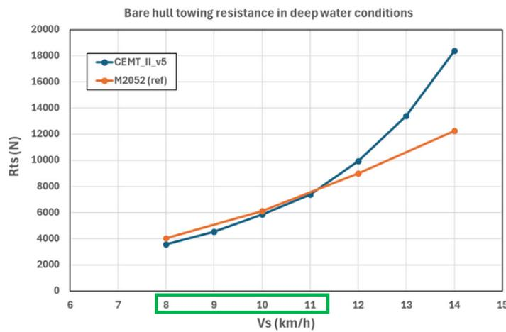
Figure 11-11: CFD bare hull towing resistance calculations in deep water conditions for the developed AUTOFLEX vessel concept (CEMT\_II\_v5) in comparison to a reference vessel (M2052 ref)
