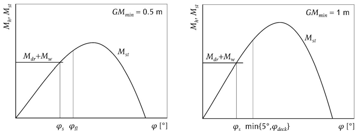
Figure 10-1: Stability criteria diagrams illustrating the righting and heeling moments for the case when containers are secured (left) and non-secured containers (right), based on [38]
