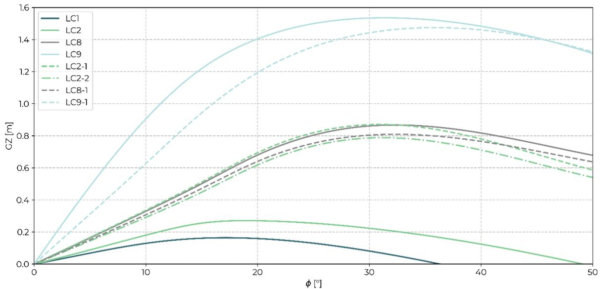
Figure 10-4: Righting lever (GZ) curves for key loading conditions (LC1, LC2, LC8, LC9) and (LC2-1, LC2-2, LC8-1, and LC9-1)
