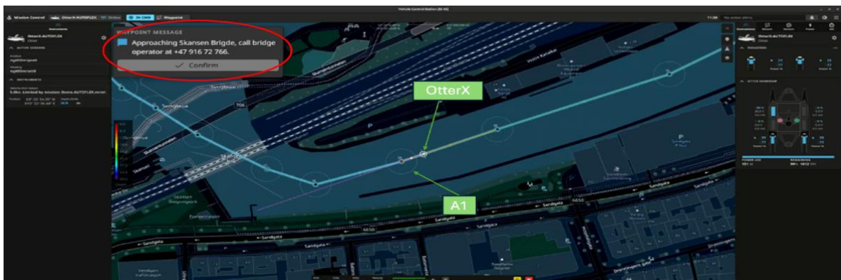
Figure 3-4: Prompt notification to ROC operator, OtterX position and action point A1
